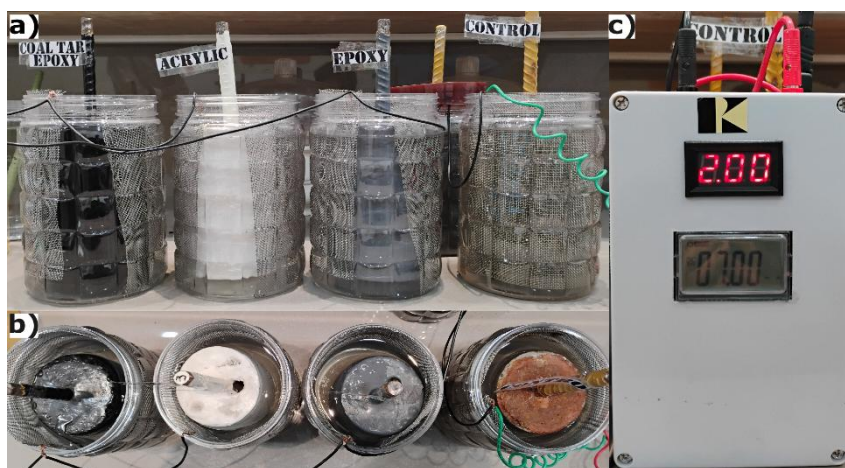
Figure 1 Accelerated Corrosion Testing of Coatings and Admixtures. a), b) Various coatings onto concrete lollipop samples immersed in 3.5% NaCl water, c) Accelerated Corrosion Testing Tool with the voltage output and current drawn displayed
